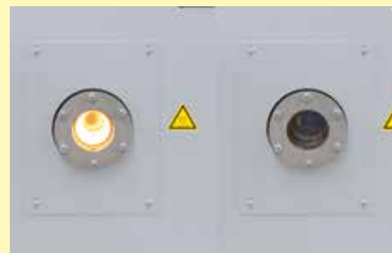
Cooled inspection glass made out of sapphire glass (left at working temperature, right at room temperature)
