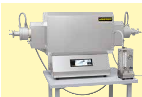
Tube furnace RHTC 80-230/16 with gas supply system 2
