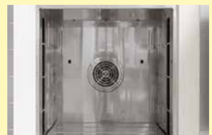
Interior made of stainless steel sheet 1.4828
