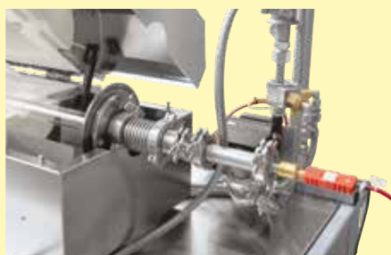
Gas tight rotating union with gas cooler and charge thermocouple
