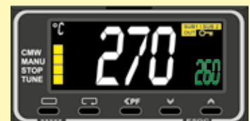
Example of over-temperature limiter
